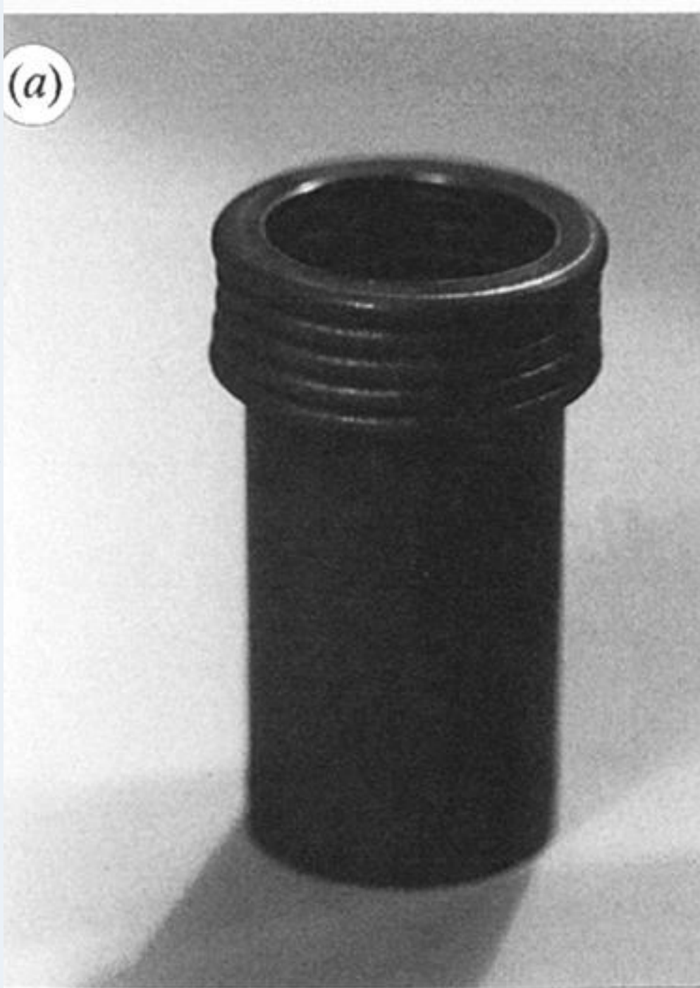
Figure 14. A comparison of crushed tubes of steel ( a ) and of woven glass cloth in epoxy resin ( b ) with V_f \approx 0.54 . The tubes are each of 50 mm diameter and of about 2.5 mm wall thickness. Each was crushed at about the same speed. Photograph courtesy D. Hull.
