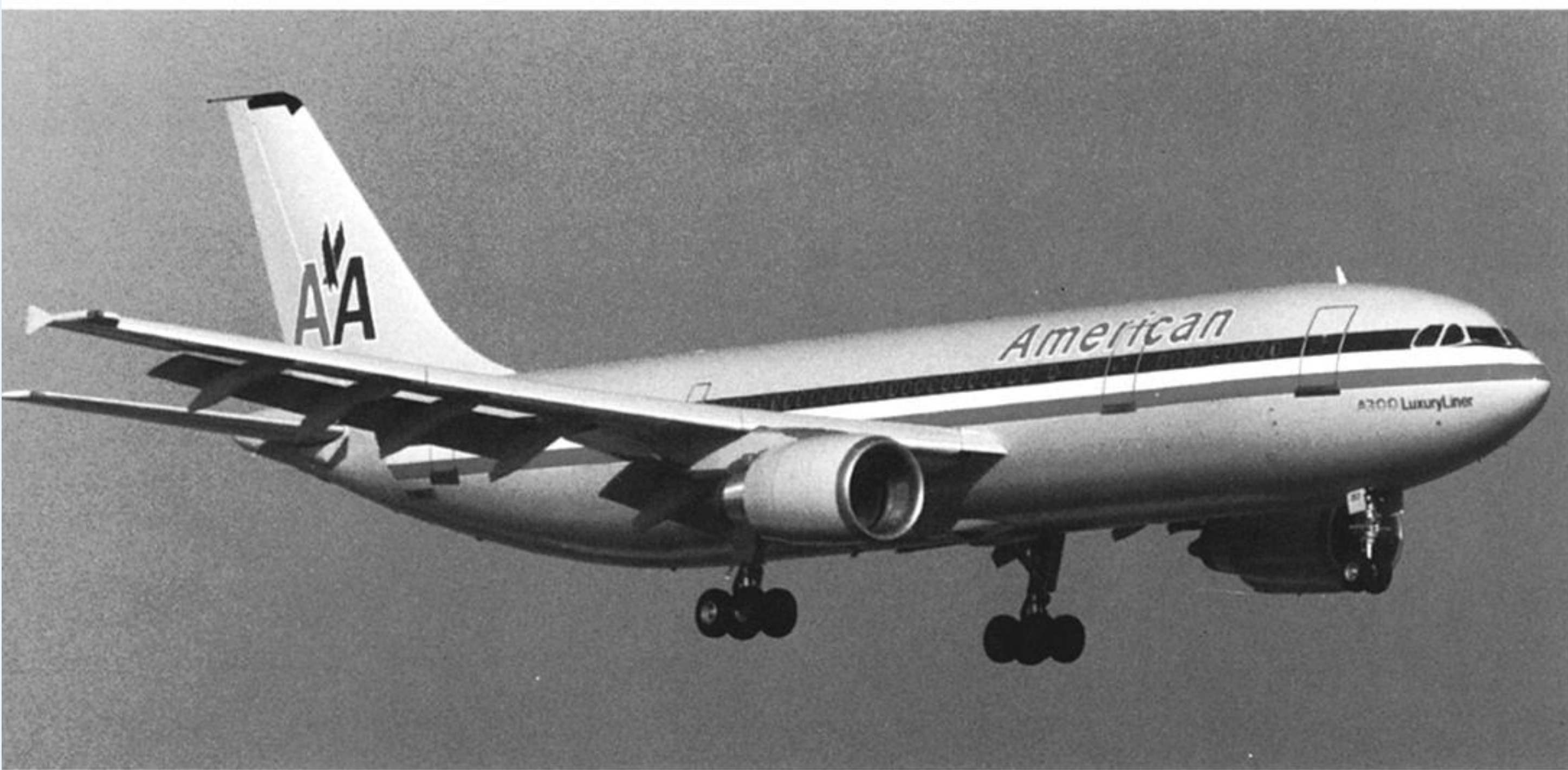
Figure 1. The Airbus A300-600, contains many components made of composites; the entire rudder and fin, engine cowlings, radome, large sections of the tailplane; the air brakes, spoilers, outer flap and wing tip, and undercarriage doors.
